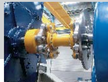
■ IXILFLEX® link type elastic coupling.
